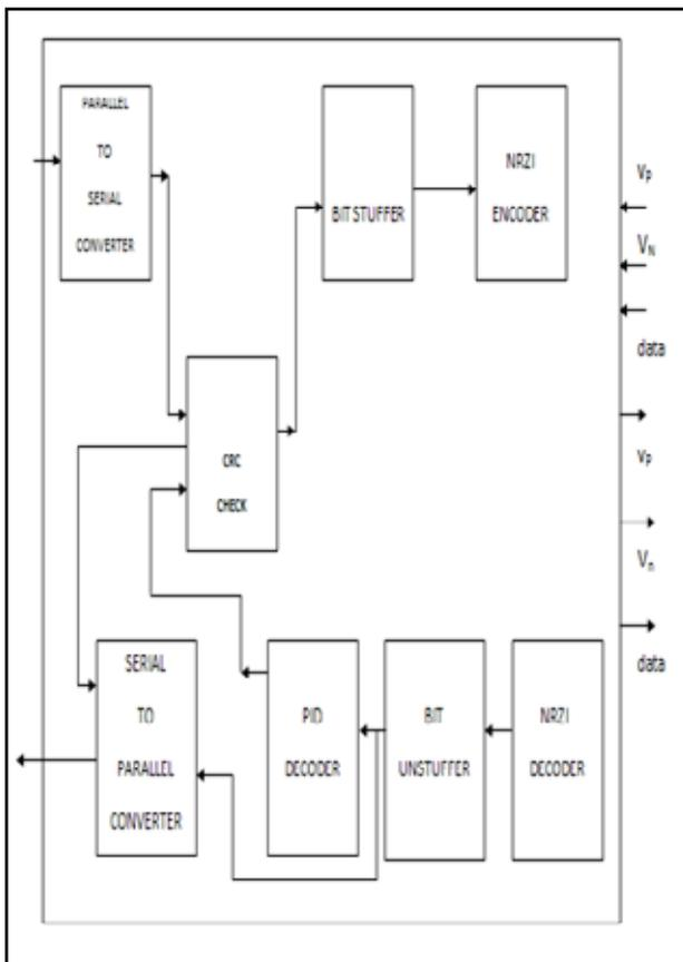
Fig. 1: Detailed Functional Block diagram
