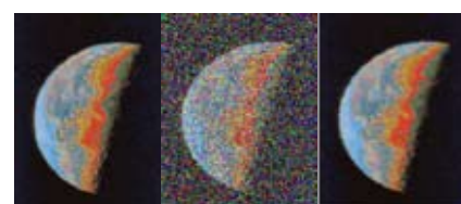
Fig. 24: Moon Image, Its Noisy Image With Salt and Pepper Noise and Its Median Filtered Images
