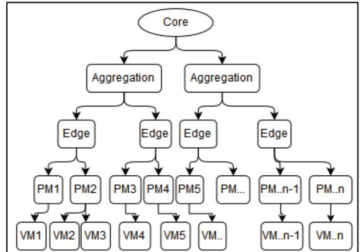
Fig. 1: Communication Network of Physical Machines and Virtual Machines
