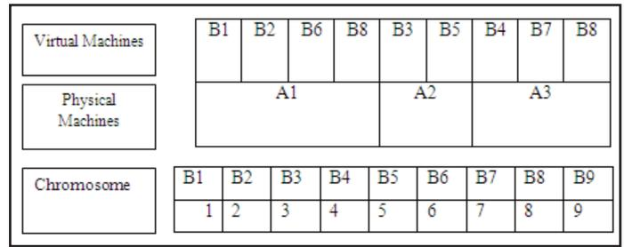
Fig. 2: Virtual Machine Allocation and its Chromosomes
