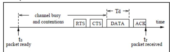
Fig. 1: IEEE 802.11 Packet Transmission
