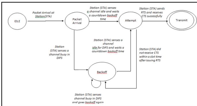
Fig. 2: State Transition of Mobile Node
