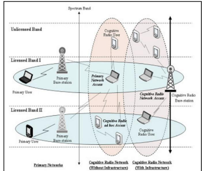
Fig. 1: Cognitive Radio System Architecture [2-3].
