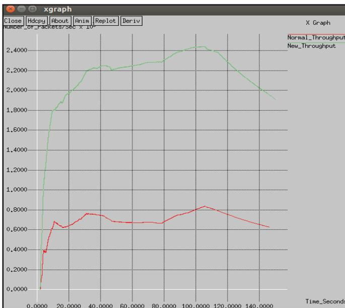
Fig. 4: Comparative Throughput Graph for Normal and Proposed New
