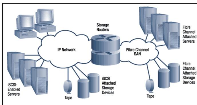
Fig. 2: Fibre Channel and iSCSI SANs Connected by a Storage Router
