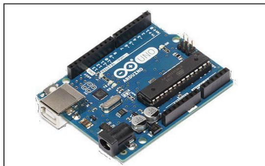
Fig. 1: Arduino UNO board
