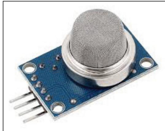
Fig. 6: MQ Gas Sensor
