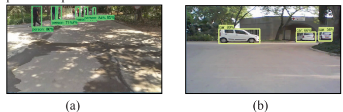
Fig. 7: Real-time Output of Classifier on Campus Road
